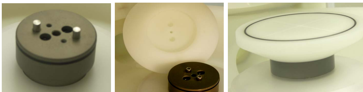
Figure 3-28 INSTALLING PRESS-ON CHUCK
