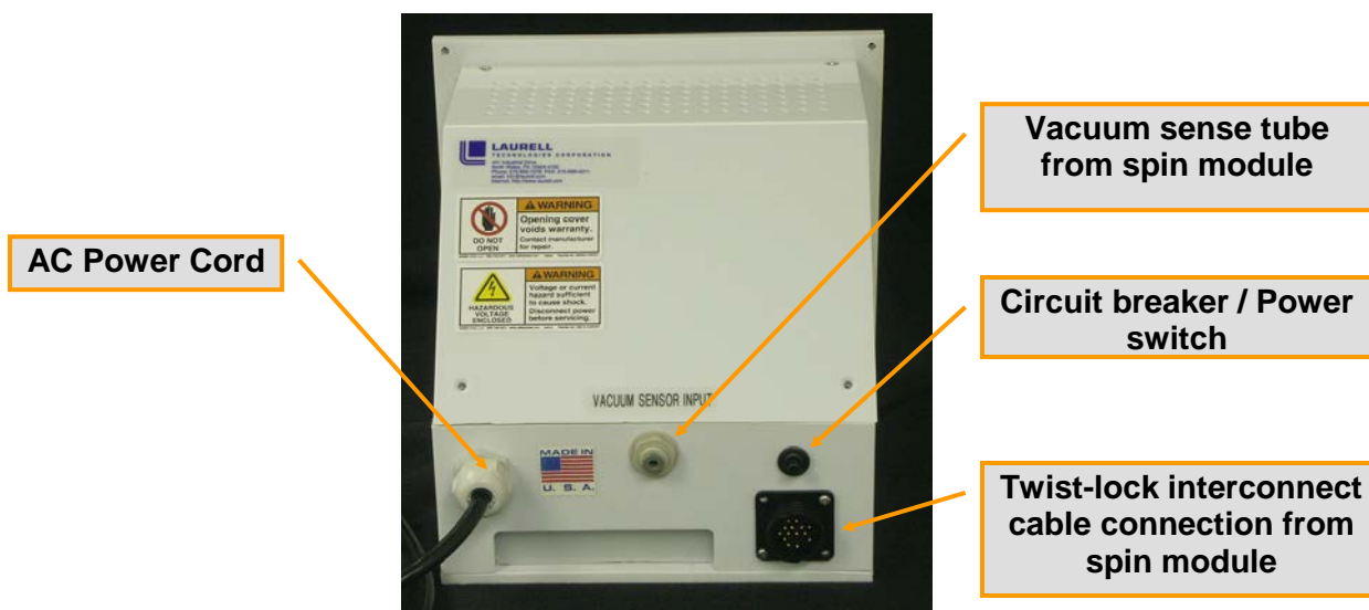
Figure 2-3A INDECK CONTROLLER – REAR VIEW
