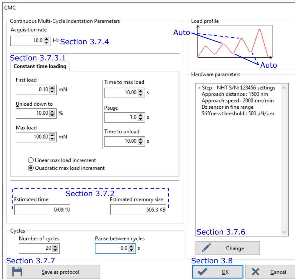
**Fig.58 CMC window parameters**
