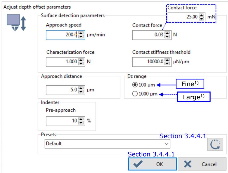
**Fig.46 MHT ADO window (e.g. default preset for hard sample)**
