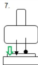
Dz sensor bridge is automatically adjusted before indentation (F)
