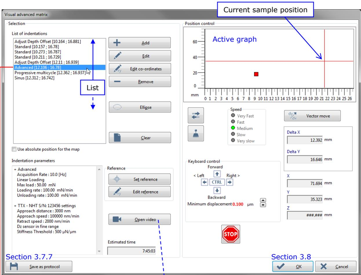
**Fig.65 Visual advanced matrix window parameters**
