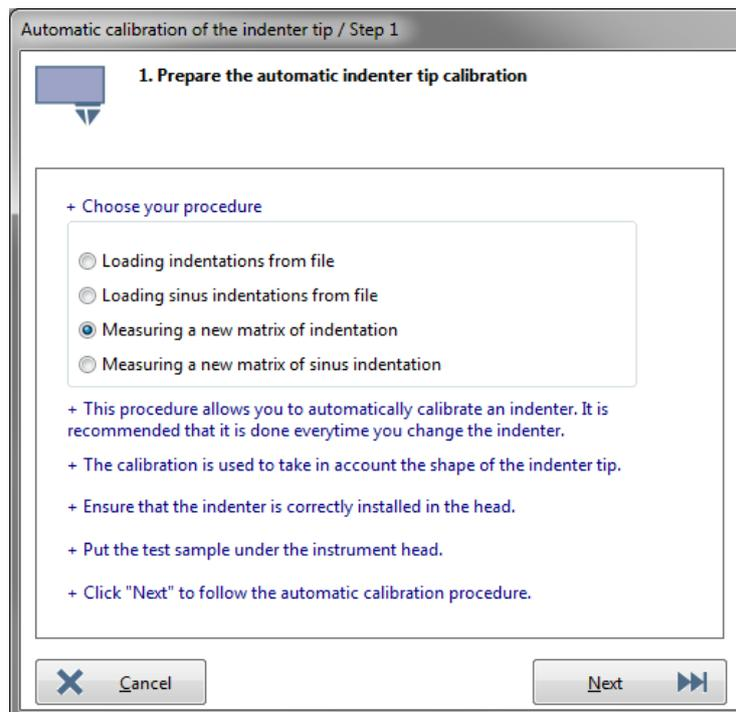
**Fig.26 Choose a calibration procedure**
