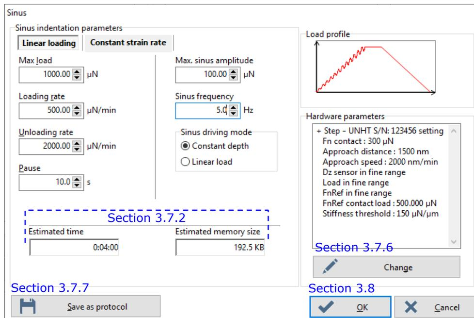
**Fig.53 Sinus window parameters**
