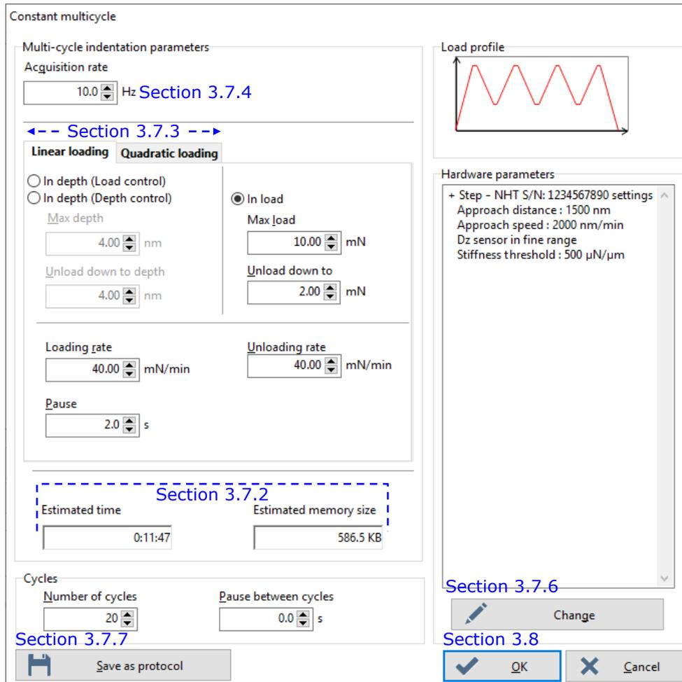
**Fig.56 Constant multicycle window parameters**
