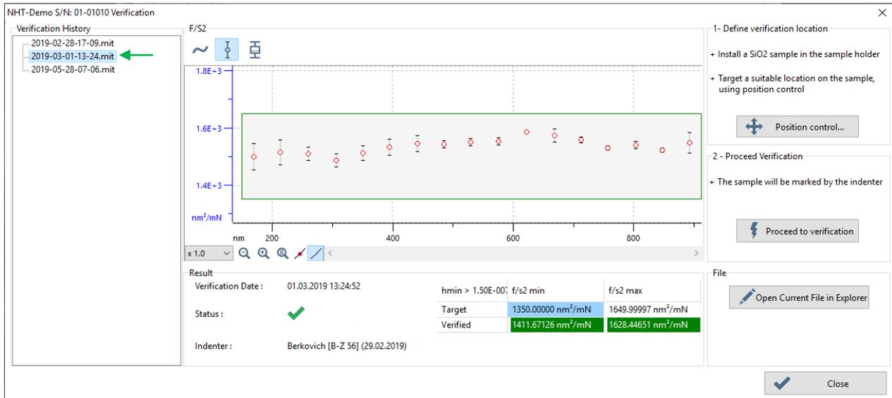
**Fig.13 Verification window - E.g. good NHT verification results**
