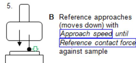
B Reference approaches (moves down) with Approach speed until Reference contact force against sample
