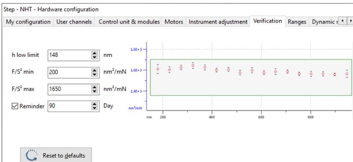
**Fig.2 Verification tab with (advised) default parameter settings for NHT**
