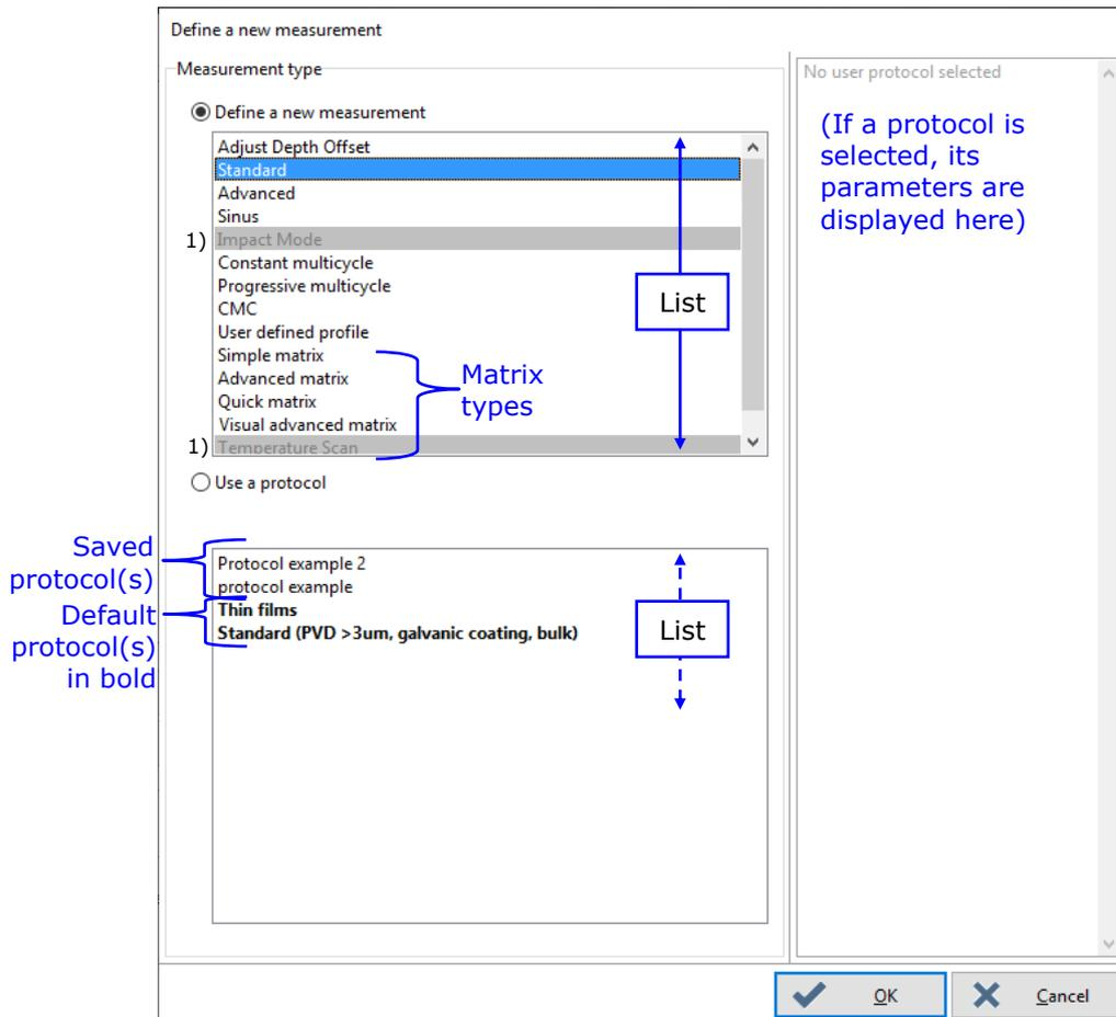
**Fig.49 Define a new measurement window**
