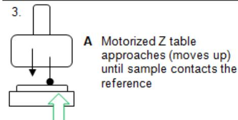
A Motorized Z table approaches (moves up) until sample contacts the reference
