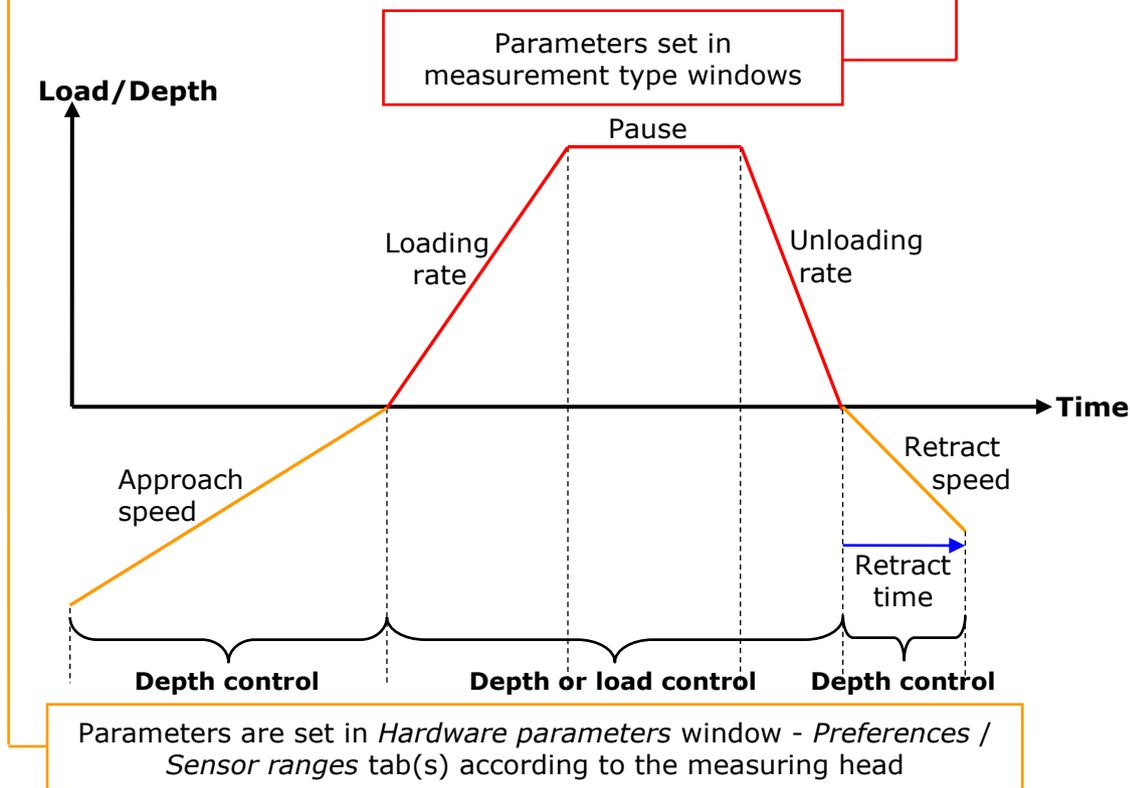
**Fig.69 Measurement schematic**
