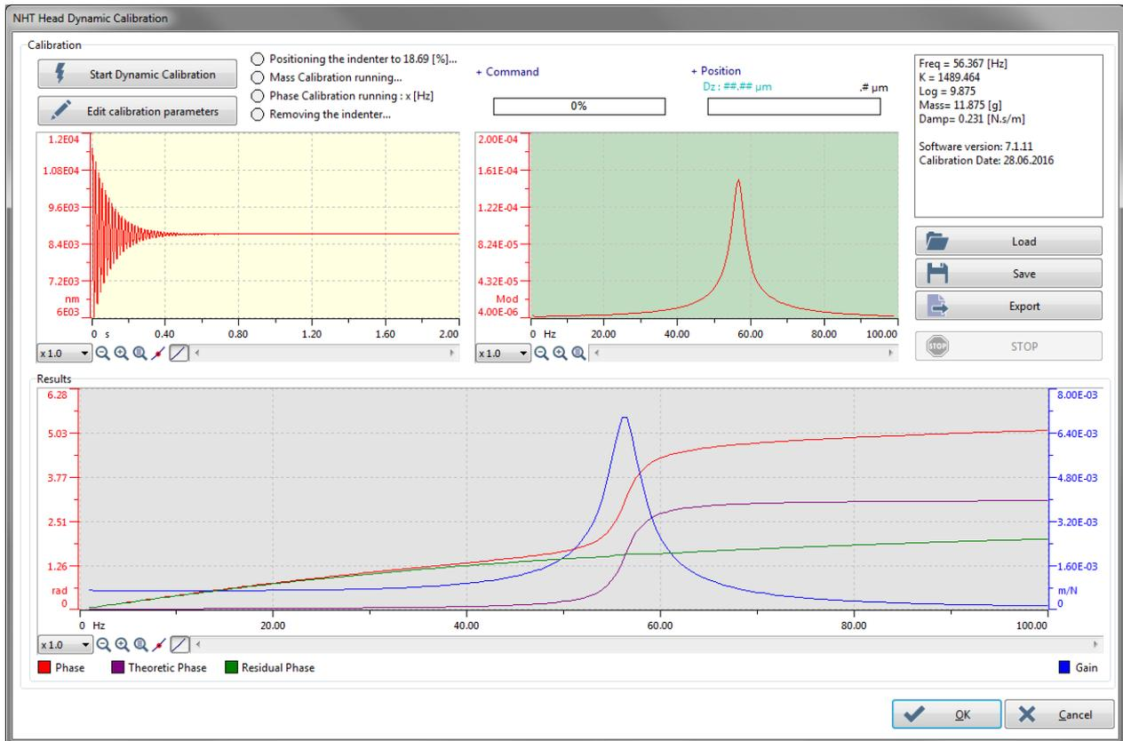
**Fig.10 Head Dynamic Calibration window (e.g. NHT)**
