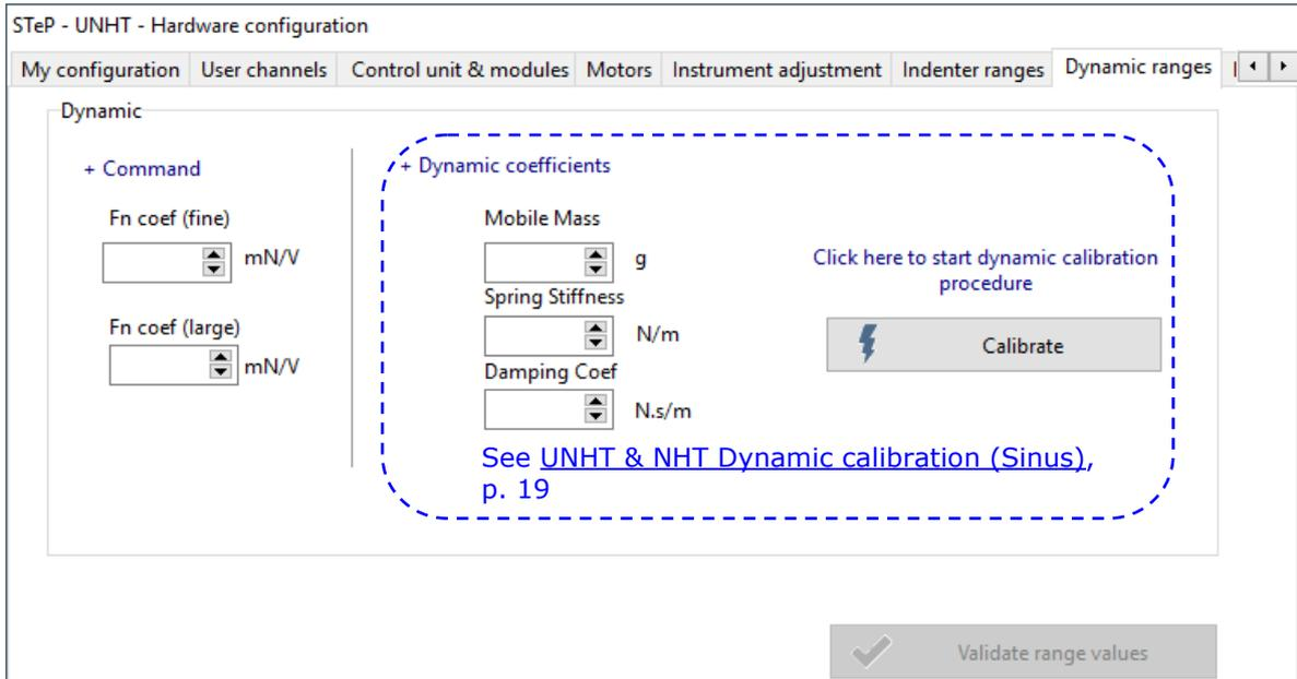
**Fig.4 UNHT Dynamic ranges tab**
