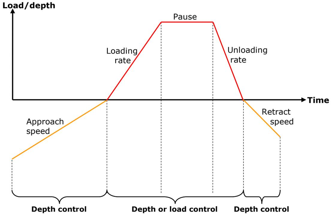
**Fig.12 Control loop schematic description**
