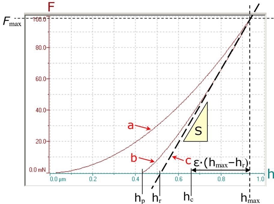
**Fig.98 Indentation test**
