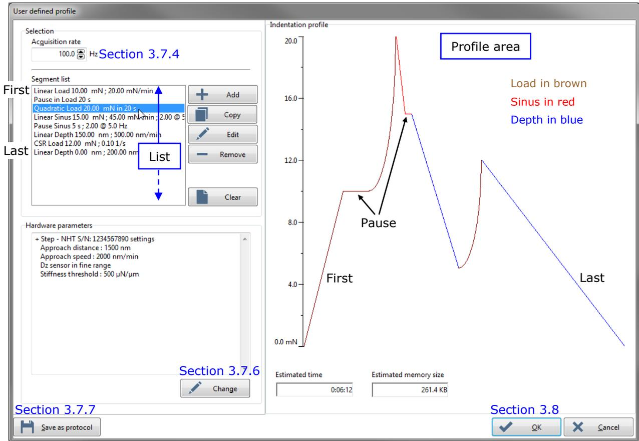
**Fig.59 User defined profile window parameters**
