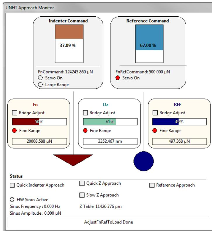
**Fig.33 UNHT Approach Monitor window**
