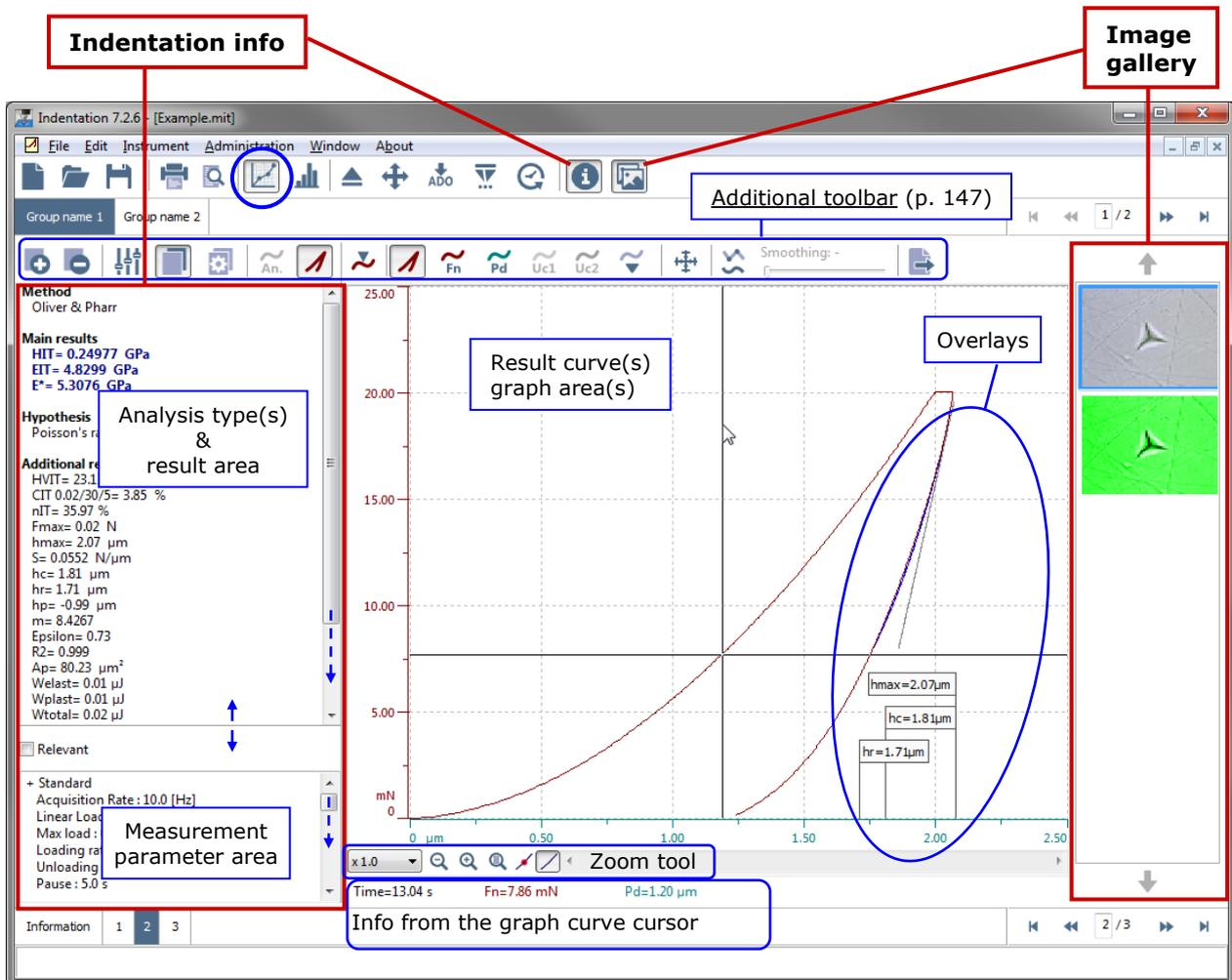
**Fig.84 Result analysis window (curve view default setting)**
