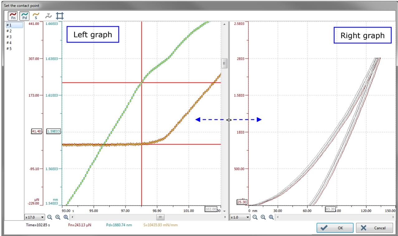
**Fig.85 Set the contact point window (default settings)**
