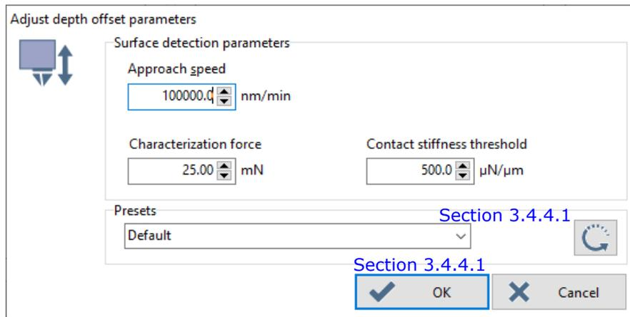
**Fig.44 NHT ADO window (e.g. default preset for hard sample)**
