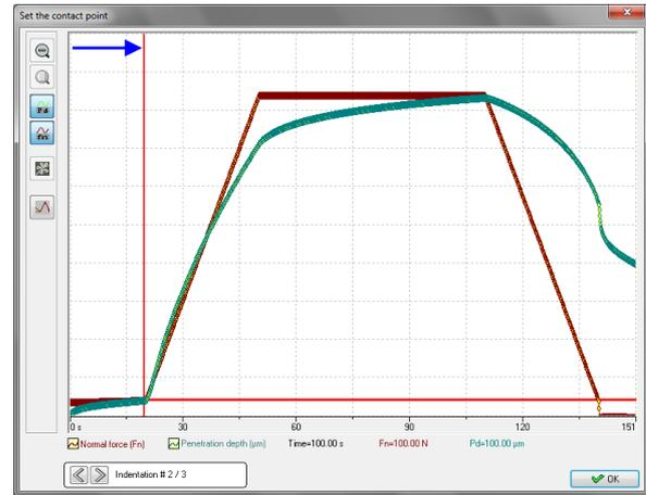
**Fig.65 Approach very short (in Set the contact point window)**
