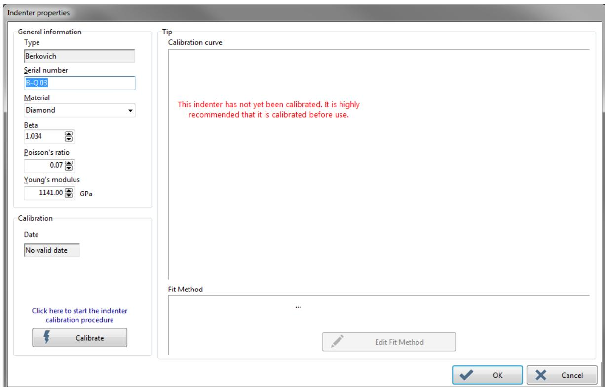
**Fig.32 Perform indenter calibration**
