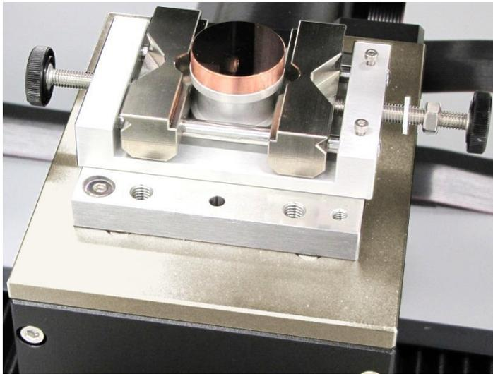
***Fig.15 Copper sample/stud solidly mounted in universal sample holder***
