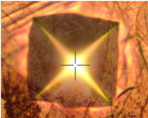
**Fig.21 Mark centered with X100 objective**
