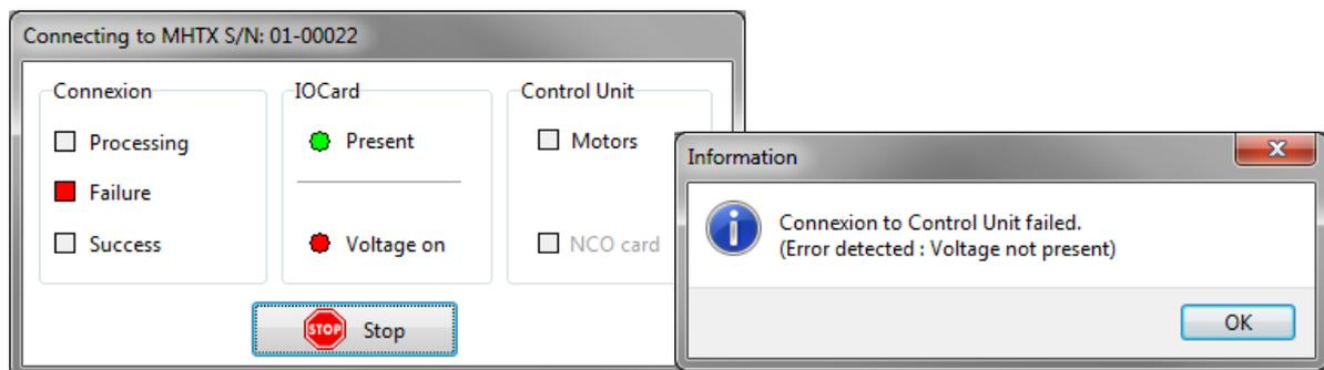
Verify that the Step is switched on (power cables plugged).
