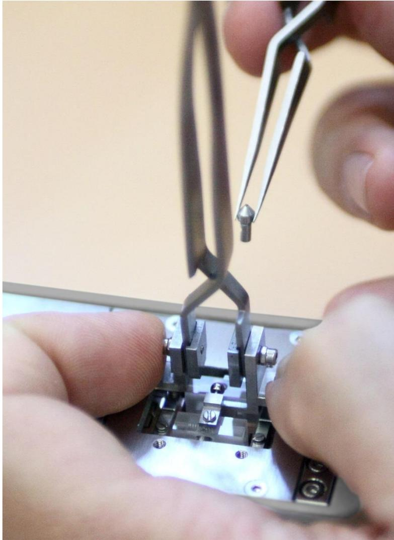
Slowly pull the indenter **vertically** up and release it; it should smoothly slide out from the glass block.
