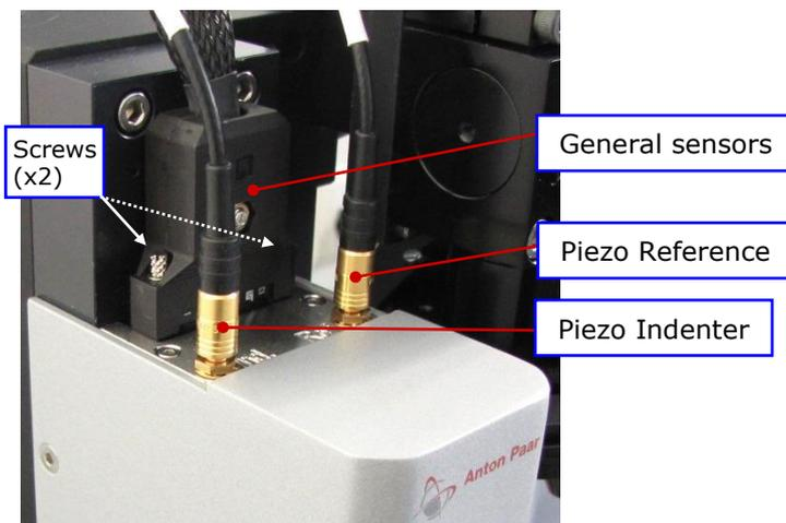
First unscrew (with a small flat screw driver) the 2 screws of the general sensors connector to release it.
