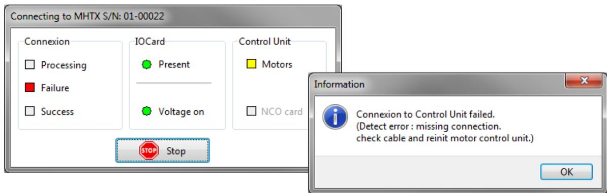
Verify that the motor cables are connected to the Step.
