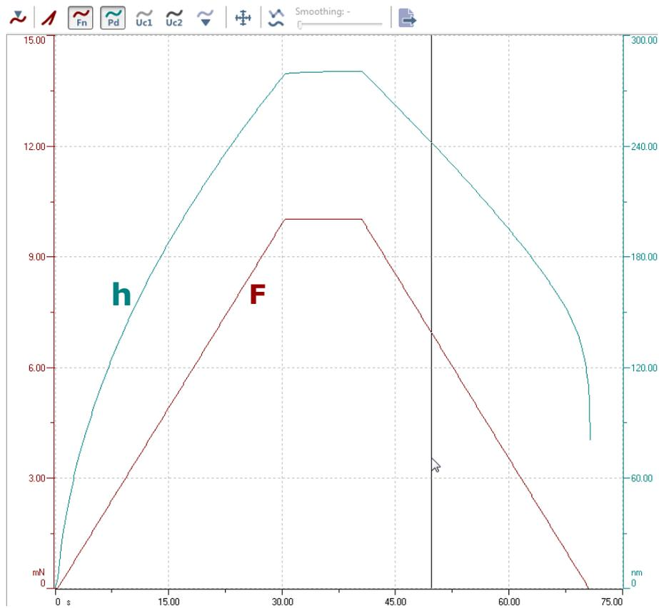
**Fig.56 Both F and h vs. time are displayed**
