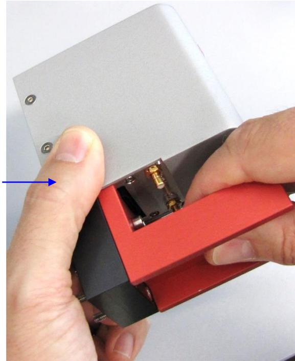
Return upside down the head by its stand and with other hand also hold the head by its rear side, near the stand (on head frame cover).
