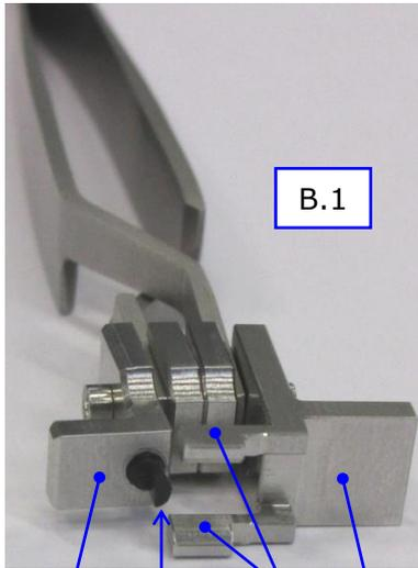
**B.1 Special (self-closing) indenter/reference exchange tool V2 (version 2)**
