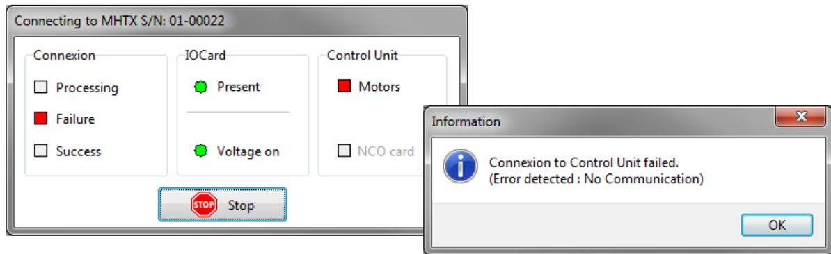
Verify that the communication Ethernet cable is connected (on acquisition system and on Step rear panels).
