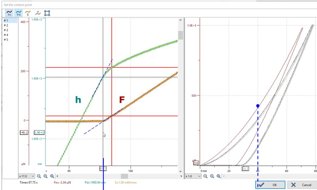
**Fig.38 Auto detect contact point**
