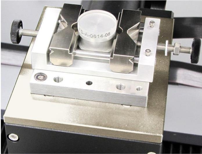
**Fig.30 Fused Silica sample/stud solidly mounted in universal sample holder**
