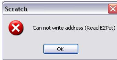
Verify that the video microscope cables are correctly plugged.
