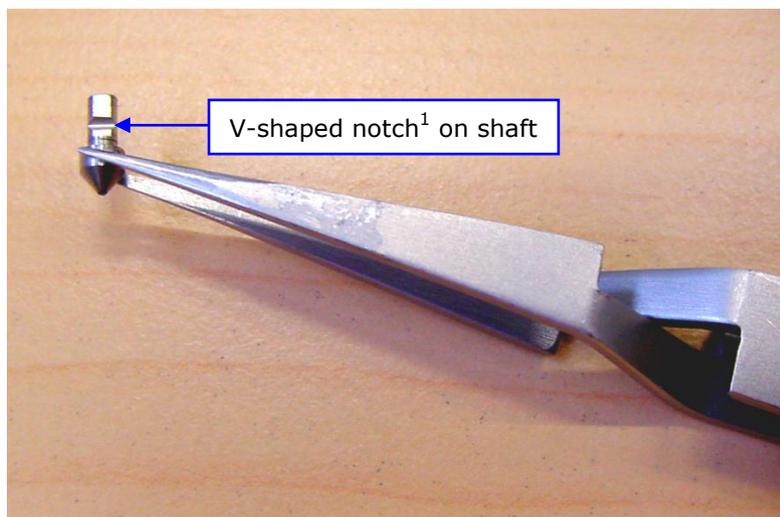
Carefully take the indenter by its head (wider part ending with the indenter diamond extremity) in the (standard) self-closing tweezers.
