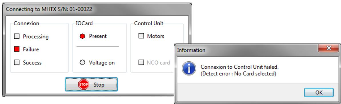
Verify that the IO card is selected ("**Instrument > Hardware configuration...**" menu bar / <Edit> button / *Control unit & modules* tab / <Choose card> button).
