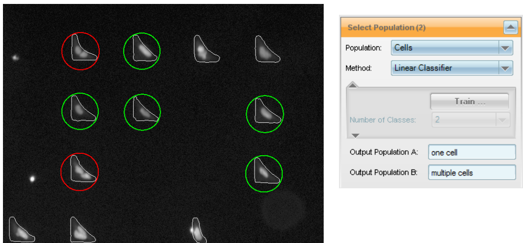
Figure 1-77: Using Select Population, method Linear Classifier to select the microstructures with one and with multiple cells. Right panel: Select Population building block. Left panel: Some selected training points shown as an overlay on the DNA stain image. Green: Population A training points (one cell). Red: Population B training points (multiple cells).
