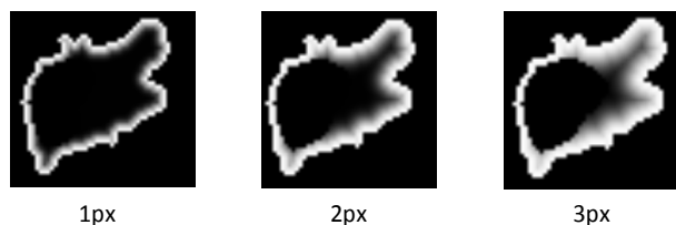
Figure 1–81: Adjustment of the STAR method’s “Profile” regions. The illustrations show an example of the Profile 1 region for three different settings of the “Profile Width” parameter. If the effect of interest is, for example, known to be confined to a region very close to the plasma membrane, a setting of 1px could be used (left panel).
