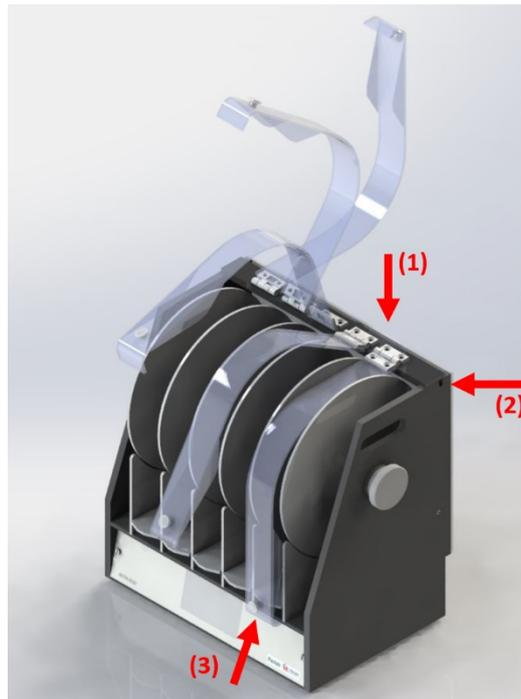
1. Standing in front of the ROTA ROD, place the cover accessory on the top of the rotarod, in line with the two lateral slots placed on the posterior part of the lateral panels – see image above (1), and pictures below.
