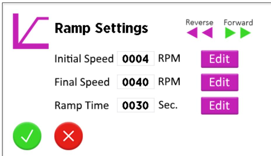
The Ramp (acceleration) is defined by 4 parameters:
