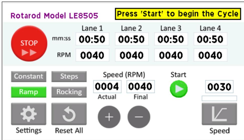
In the **Held** state, the message “Press ‘Start’ to begin the Cycle” is displayed, meaning that the unit is waiting for the user to press the **Start** button for initiating the speed ramp/acceleration. In the meantime, the speed of the rod is maintained to 4 rpm.
