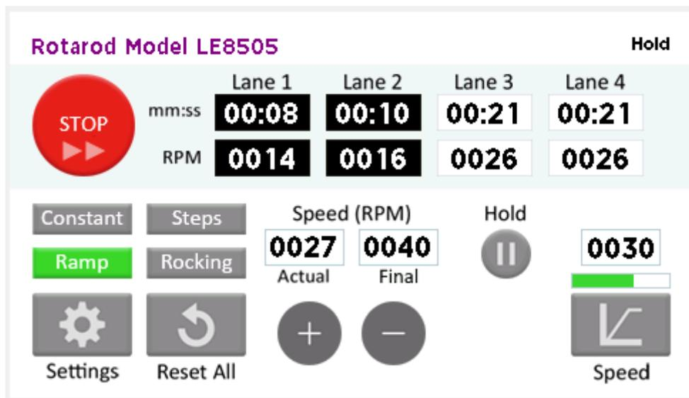
When pressing the **STOP** button, the ROTA ROD switches from the **Hold** to the **Waiting** state and the motor stops rotating.
