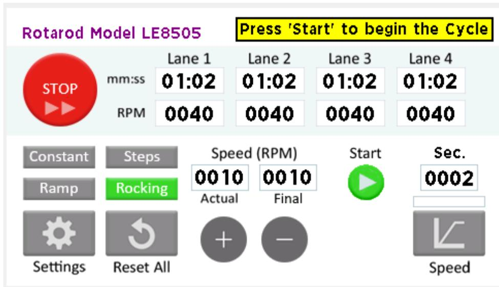
The speed of the rod is constantly maintained at the Initial Speed of the first Step and the message “Press ‘Start’ to begin the Cycle” is displayed, meaning that the unit is waiting for the user to press the **Start** button for initiating the user-defined speed protocol. In the meantime, the speed of the rod is maintained to 4 rpm.
