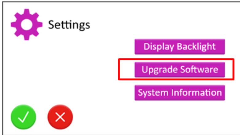
**NOTE:** To exit boot loader mode without upgrading the software, power cycle (restart) the control unit.
