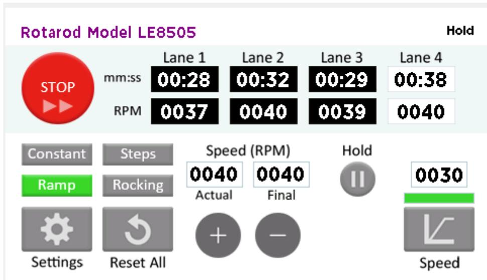
If the **Hold** button is pressed during the ramp/acceleration process, the ramp/acceleration is interrupted, and the rod will continue to rotate at last speed value.
