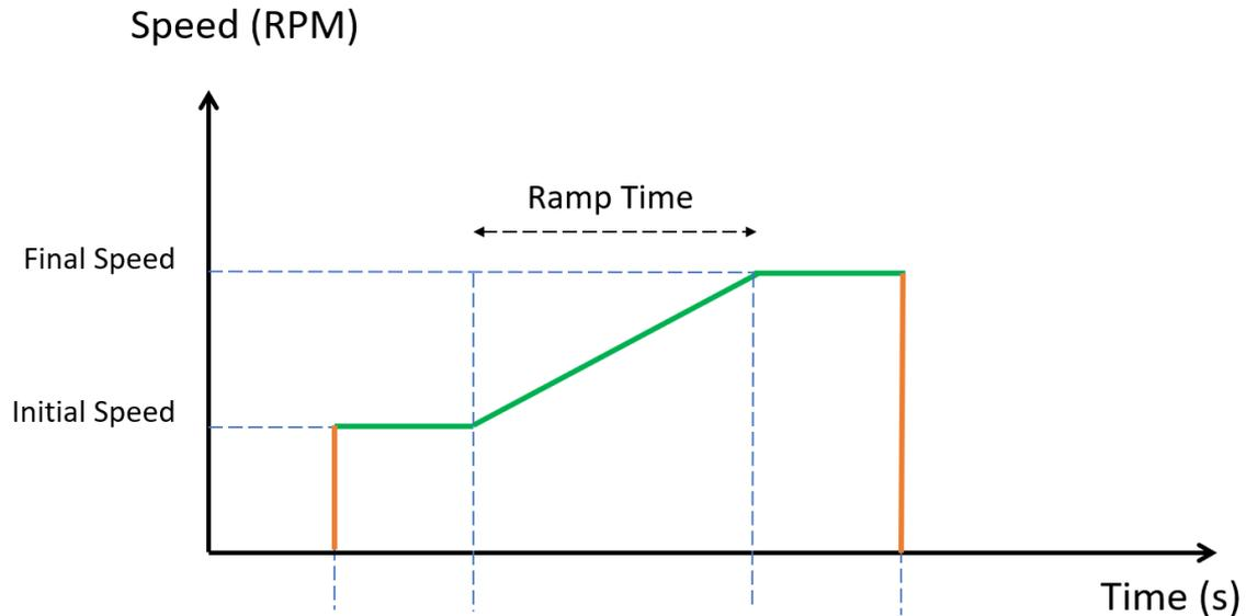
If the Initial Speed is lower than the Final Speed, the speed is accelerating.
