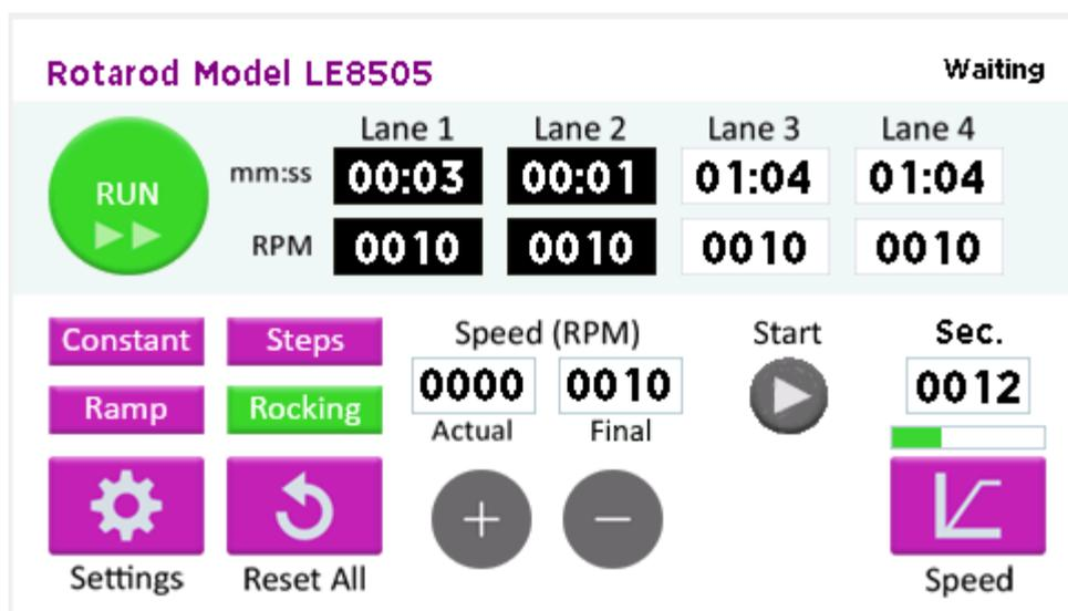
To select the ROCKING working mode, press the **Rocking** button. The button of the selected working mode will highlight in a green color.
