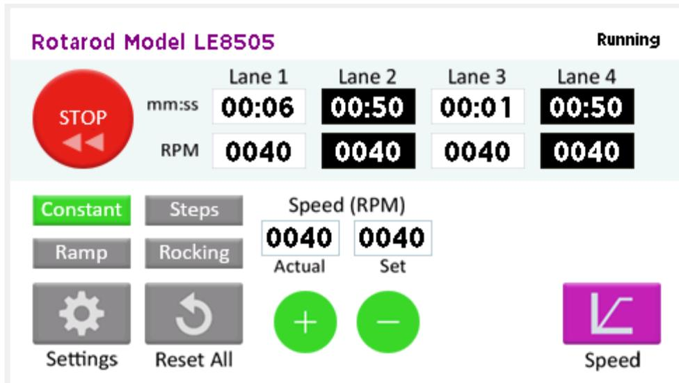
While running, the speed can be manually changed by the user by using the green + and – buttons available on screen.
