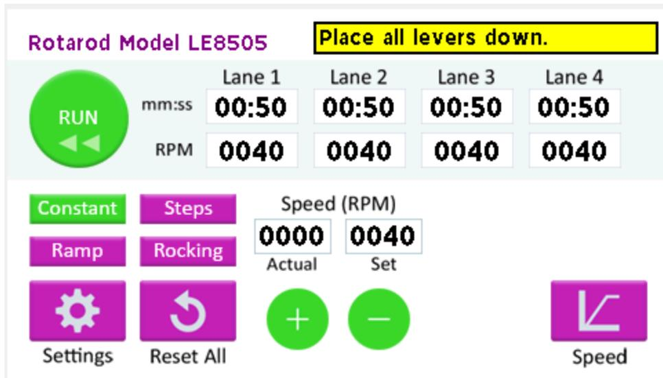
In the **Waiting** state, when the levers are in the down position, the counters of the inactive lanes are displayed in white text on black background colour.
