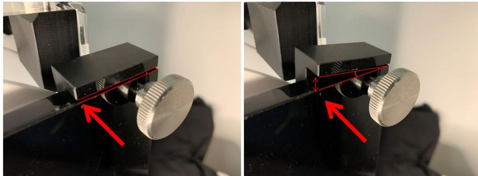
2. Maintain the cover in place by tightening the 2 lateral screws provided with this accessory. – see image above (2)
