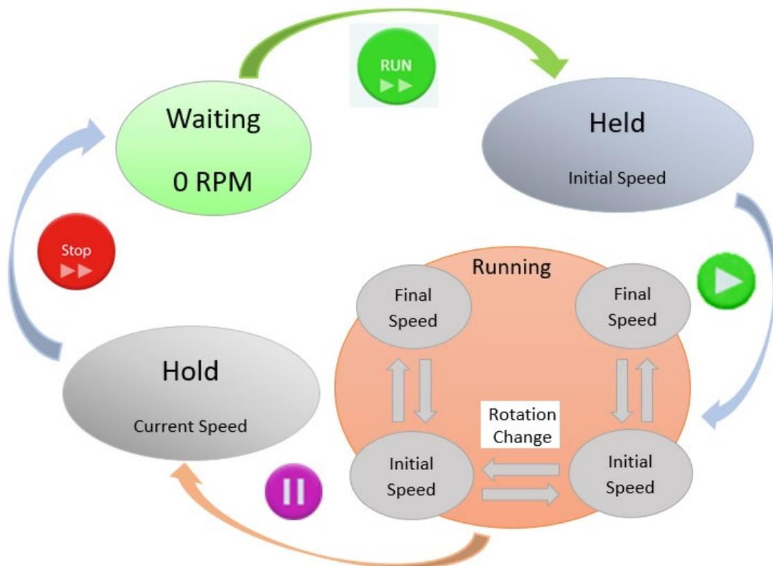
In the **Reverse Ramp Rotation** protocol, the initial speed is different than the final speed.
