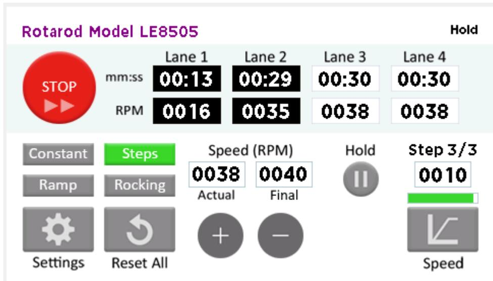
Once the Ramp Time is elapsed in the last step of the protocol, the speed of the ROTA ROD is constantly maintained at the Final Speed and automatically switches to the **Hold** state.
