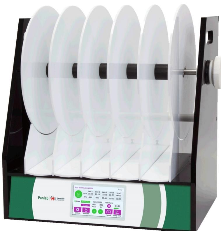
In operation, the animal is placed on the rotating lane of the ROTA ROD and the timer is started. When the animal drops safely into its own lane, the latency time to fall (minutes and seconds) and final rotation speed are automatically recorded.
