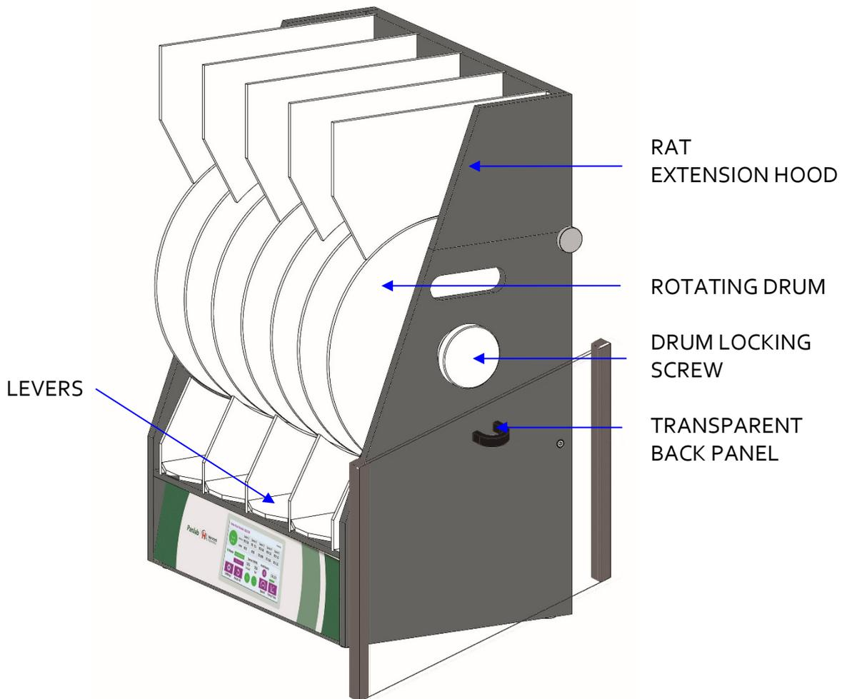
The ROTA ROD LE8305 (76-0771) and the LE8505 (76-0772) have a rotating rod with 4 lanes. The LE8205 (76-0770) features 5 lanes and the LE8355 (76-0773), 2 lanes. Rodents (rats or mice depending on the instrument model) are placed in individual lanes, on the top of the rod. There is a transparent wall fixed with magnets to the rear side of the ROTA ROD to prevent any animal escape from the posterior side of ROTA ROD.
