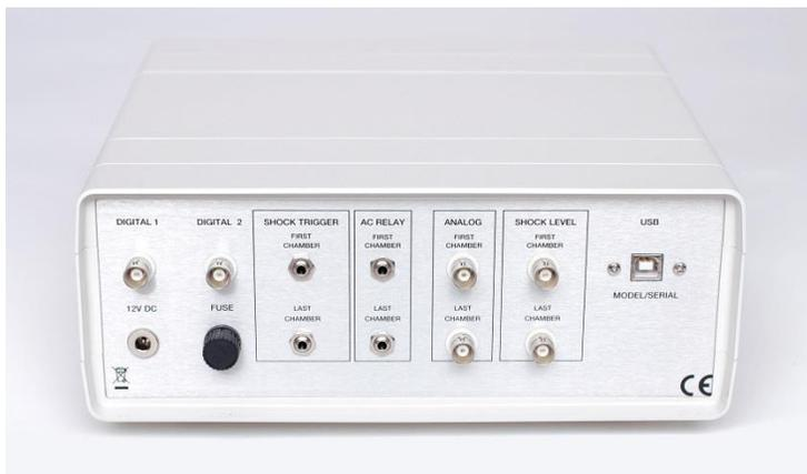
Connect Shock Trigger First Chamber to Remote Operate + on the back of the first shocker. Run a trigger cable from Remote Operate – on the first shocker to Remote Operate + on the second shocker. Continue this pattern until you go from Remote Operate – on the last shocker to Shock Trigger Last Chamber on the control box.
