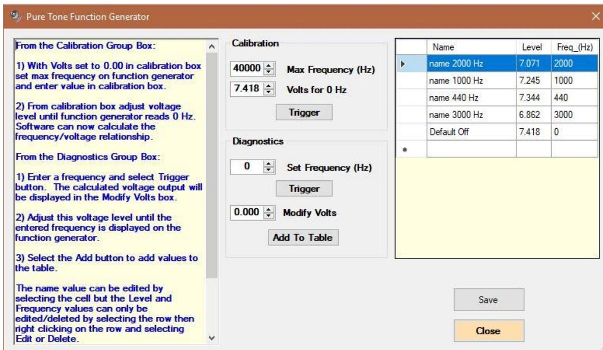
In this window there are instructions for calibrating and setting up pure tone frequencies. The best default is to set the function generator range set to 50k and output to sine ( $\sim$ ).
