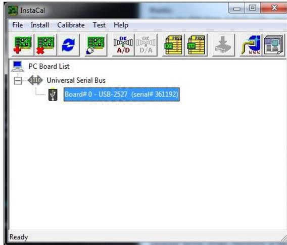
7. Once the board is recognized Board#0 - USB-2527 (serial#.....). Write down this serial number and keep it in a safe place.
