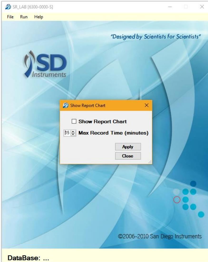
This is an example of a trial definition using extended record time. This trial example starts recording data at time 0 and then the ACR is turned on at time five minutes. Then, five minutes later (time at 10 minutes) turned off. All Stimuli can be incorporated in an extended time trial definition including Background, Analog and all Cue Out Stimuli.
