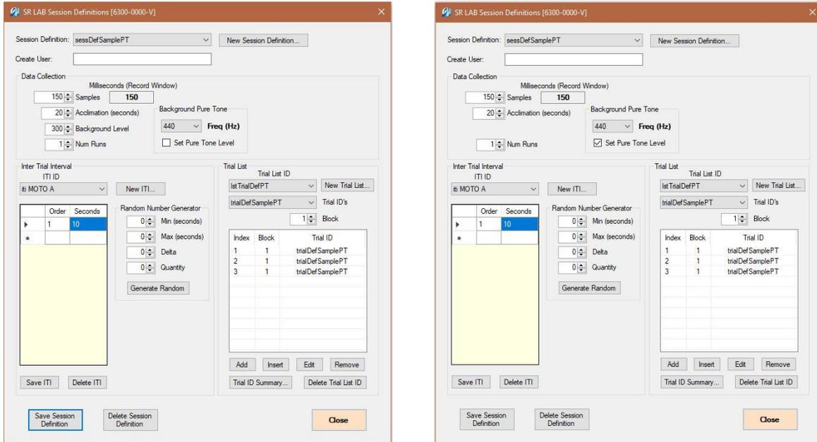
To select a pure tone background, select a frequency from the dropdown box and check the Set Pure Tone level. This will hide the white noise background and set its value to 0 volts.
