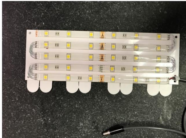
Note: On the white light the tabs of 3M Command® strips which are pulled down to remove the light bar.
