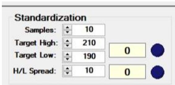
**NOTE:** Animals of different sizes may require an increase or decrease in amplification to obtain normal data. The user may adjust the response gain (amplification) as high or as low as the dial will allow, to a level suitable for their needs, and establish new standardization values based on these. It is important that the calibration value is equal across all SR-LAB cabinets.
