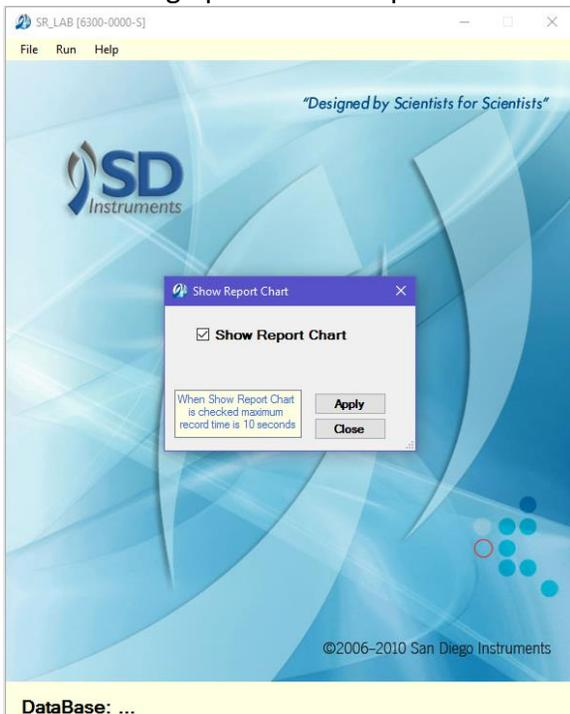
When the Show Report Chart checkbox is checked the maximum record data time is 10 seconds (10,000 msec). When this checkbox is unchecked there is an additional parameter that allows the user to extend to the time from 1 minute to 30 minutes with a one minute resolution.
