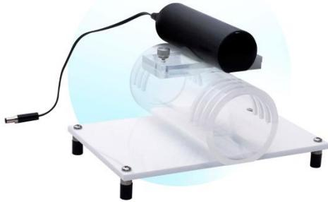
5. Plug the power cord into the power jack. On newer units there is a power jack in the ceiling at the front. On other units the Aux Power jack on the side of the cabinet is used. If using the cable to the Aux Power jack on the side of the test station drape it over the top of the cabinet to remove the weight of the cable.
